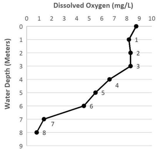
**Figure 4** Dissolved oxygen data sampled at 1-meter intervals. Average of 8.38 mg/L between 0 to 3 meters followed by a precipitous decline to 6.62 mg/L at 4 meters. Oxygen levels continue to drop to 0.8 mg/L at the bottom of the lake. Data collected 9/2017, Lake Pontoosuc, MA.
